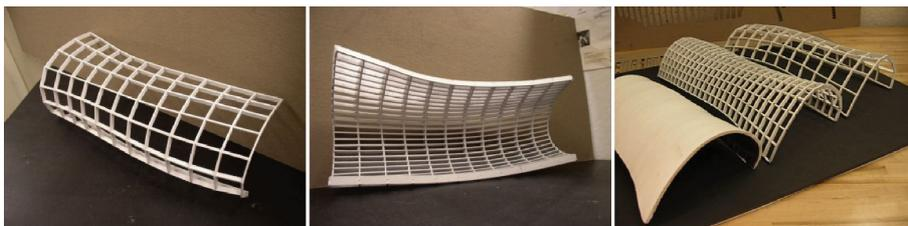
Figure 1. Assembled prototypes with various rib densities.
