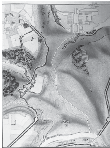
Figure 1: Hatching following the lines of curvature of the surface Dalesme's portfolio, 1812. Exercise at the Ecole polytechnique
